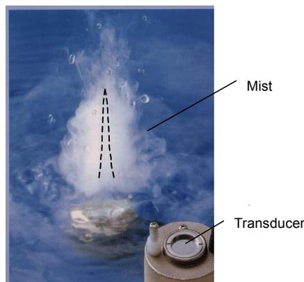
Fig.1 Ultrasonic atomization and ultrasonic transducer.
