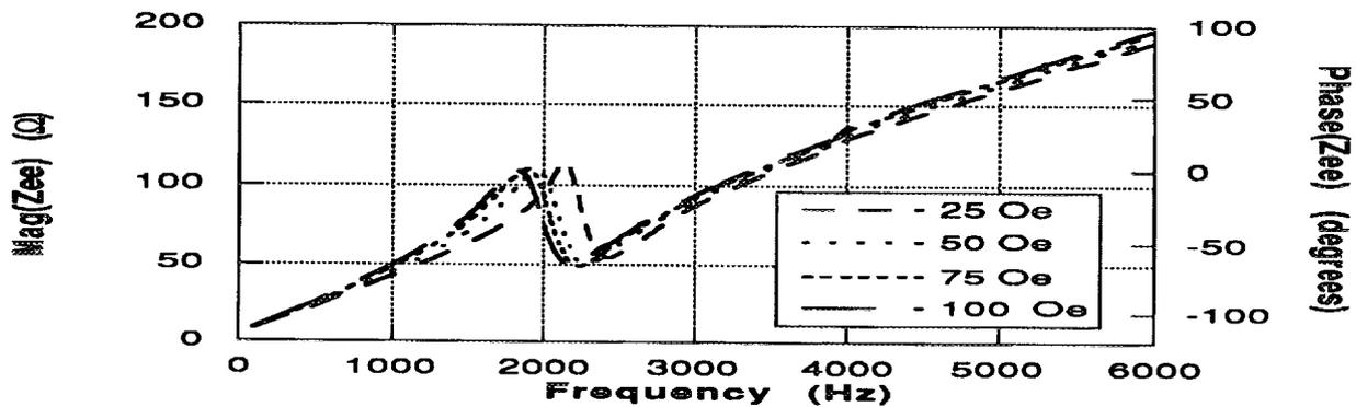
FIGURE 3. Electrical impedance functions reflecting shifts in resonance and anti-resonance frequencies with operating conditions. The frequency of maximum efficiency decreases slowly with the changes in electrical impedance anti-resonant frequencies, while the system mechanical resonance decreases more rapidly with changes in the electrical impedance resonant frequencies.
