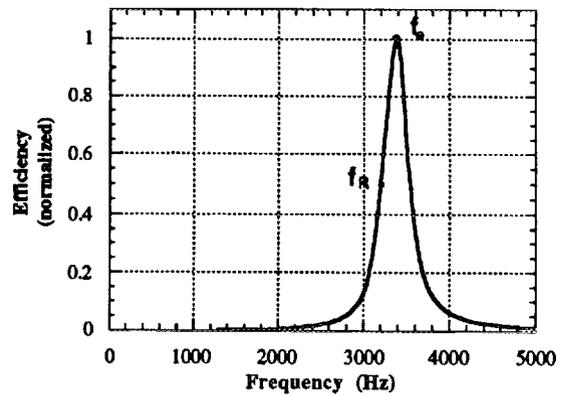
FIGURE 2. Normalized efficiency versus frequency measured as the mechanical output supplied to the load over the electrical input into the drive coil.
