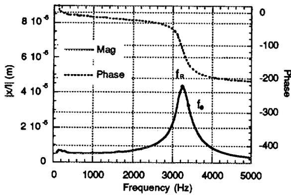
FIGURE 1. Displacement per current calculated from the acceleration output at each frequency.  $f_R$  is approximately the frequency of the mechanical resonance,  $f_E$  is the frequency of maximum efficiency.
